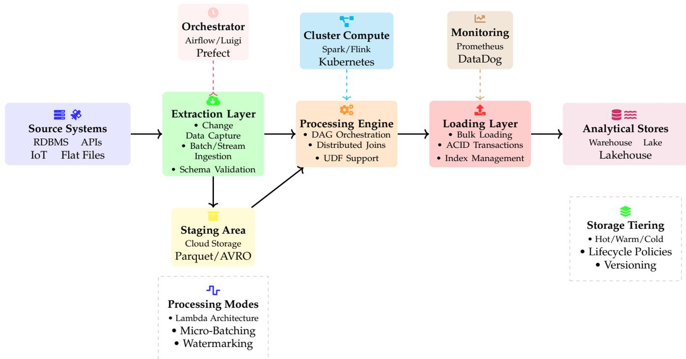
**Figure 3.** Enterprise ETL Architecture with Centered Alignment and Enhanced Connectivity
